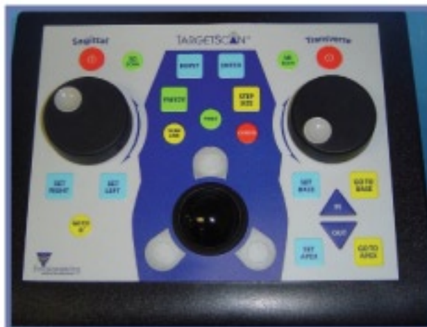
The control box allows physicians to move the scan plane back and forth while the probe remains stationary.
